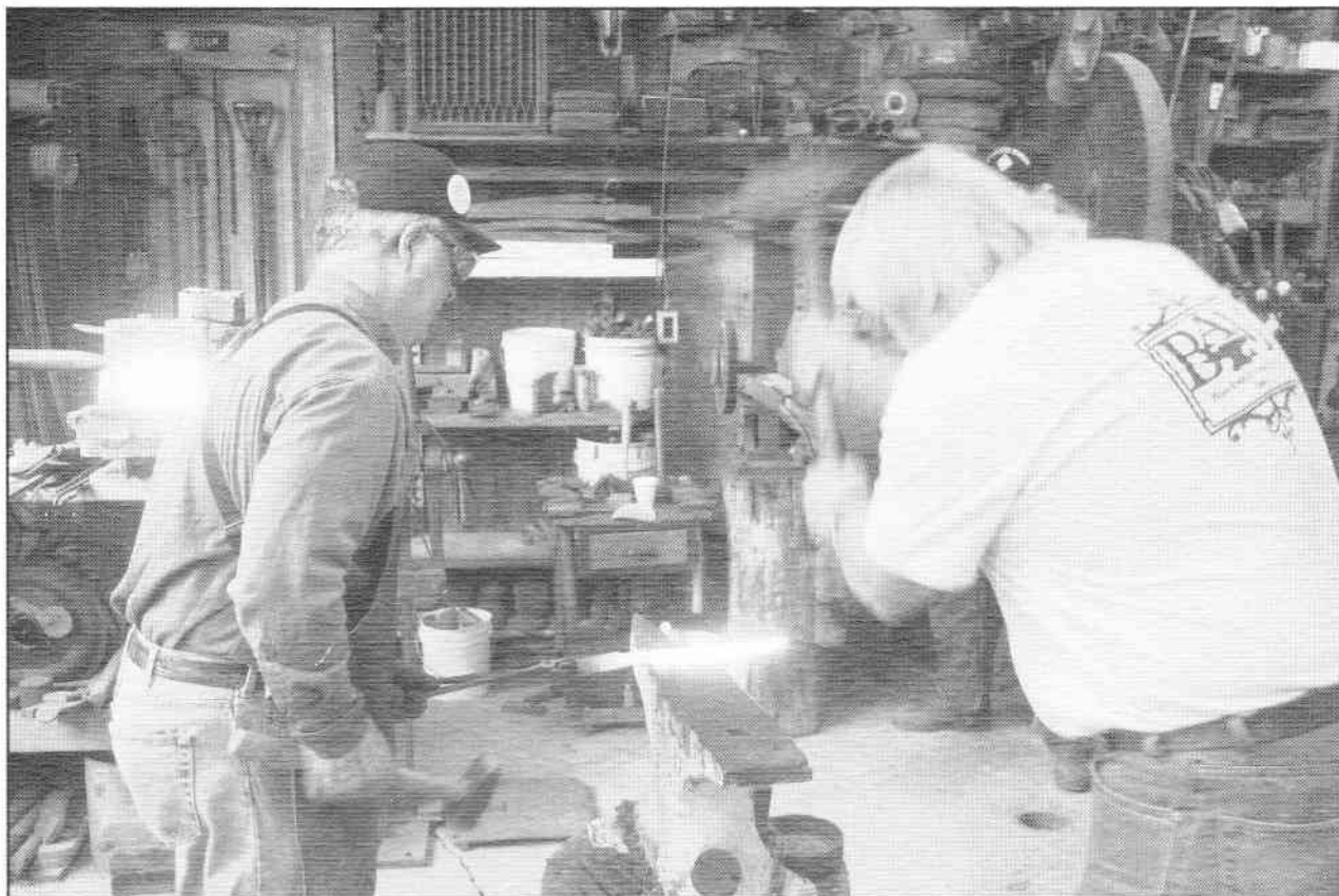
V.J. McCrackin gets some help from human power hammer Bob Stormer as he draws out the whale skinner he forged for the November BAM meeting.
