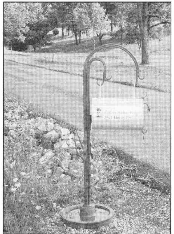
Don't think I ever ran a photo of my new mailbox in the newsletter so here it is. Base is a tractor wheel, box is 3/8 thick walled pipe, support 4 pieces of 5/8 inch round welded together. I made weeds to go around the base.
