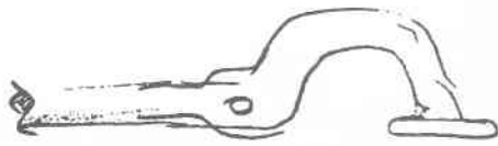
JAW ON T. USED TO GRIP ASHTRAY STOCK.
