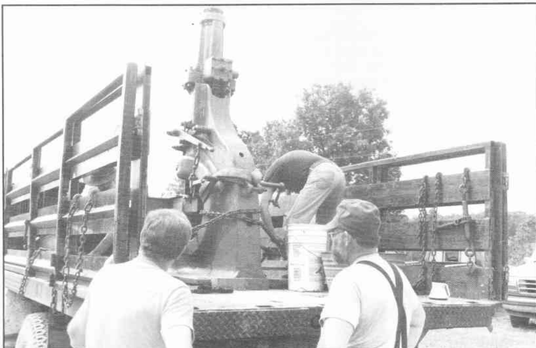
Above: May meeting demonstrator Bill Miller welds a Damascus billet on Ray Chaffin's new hydraulic forging press. The press still had a little wet paint but Ray got it together just in time for the meeting. Bill proved an excellent knifsmith. Below: Ray admires his new toy while trying to figure out how to get it unloaded.
