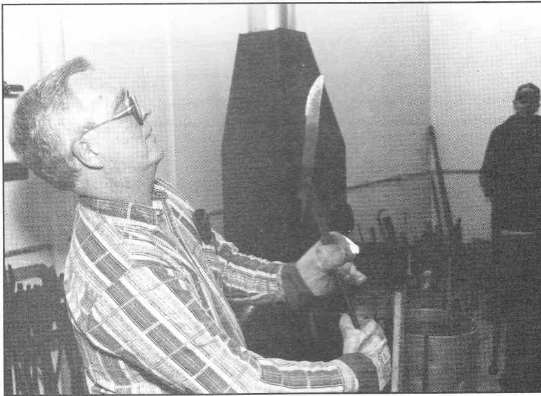
Left: Bladesmith V.J. McCrackin stepped up to the forge and knocked out a quick blade from a piece of spring.
