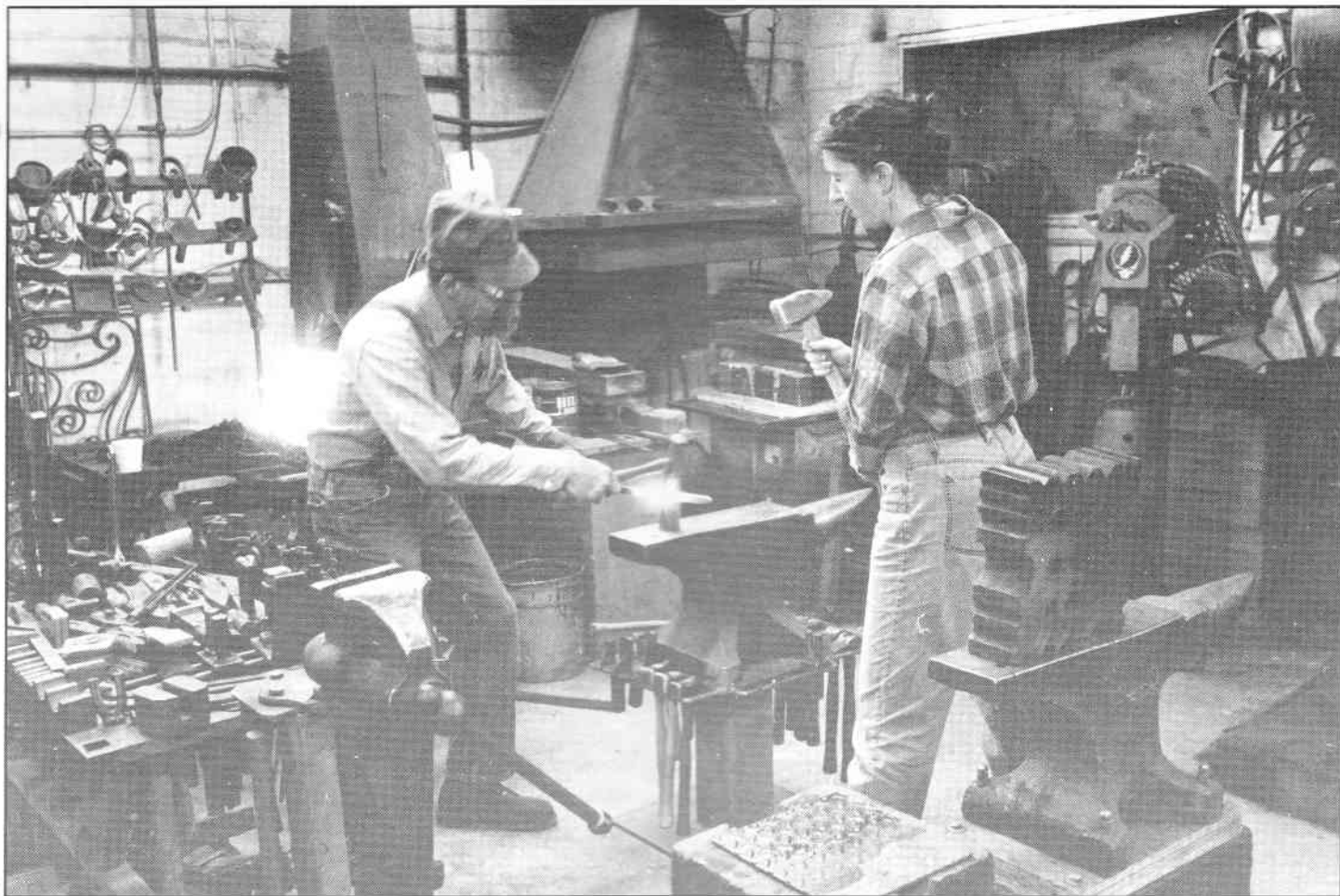
Above: Walt Hull and Kate Dineen teamed up to show us how to forge a diamond on the diamond balluster from 5/8 inch square stock.
