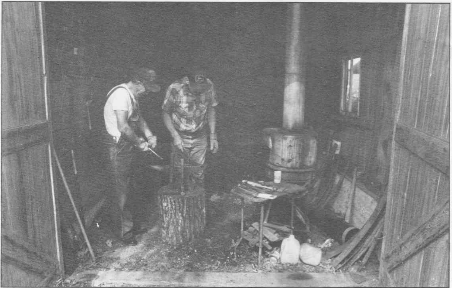
Paul Martin, left, and Ray Joe Hastings teamed up the past year to learn gigmaking, an Ozark tradition that dates back three generations in Paul's family. The two spent many mornings in Paul's Bunker, Mo. shop forging gigs from leaf springs using only the simplest of tools. It's hard work but Paul makes it look easy and Ray is learning fast.
