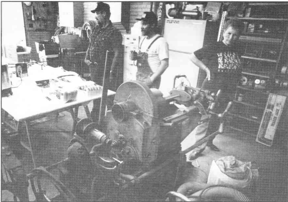
Left: Everyone had to admire Jim Kendzora's cold twisting machine which could twist 1/2-inch square with the flip of a switch. It also untwists.
