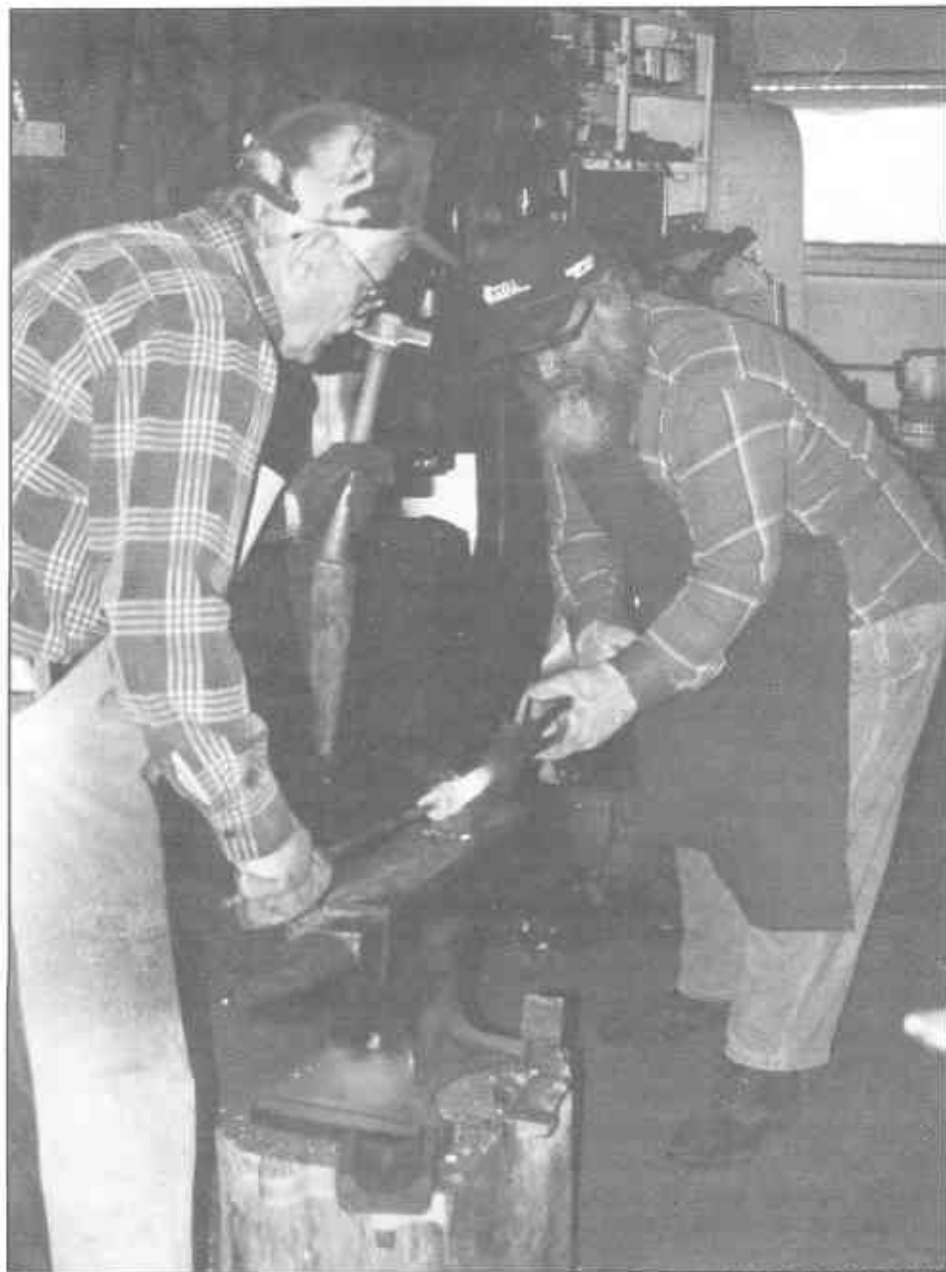
Right: Guy McConnell, left, and Bill Briggs weld toward the end of the Damascus pistol barrel they are building.
