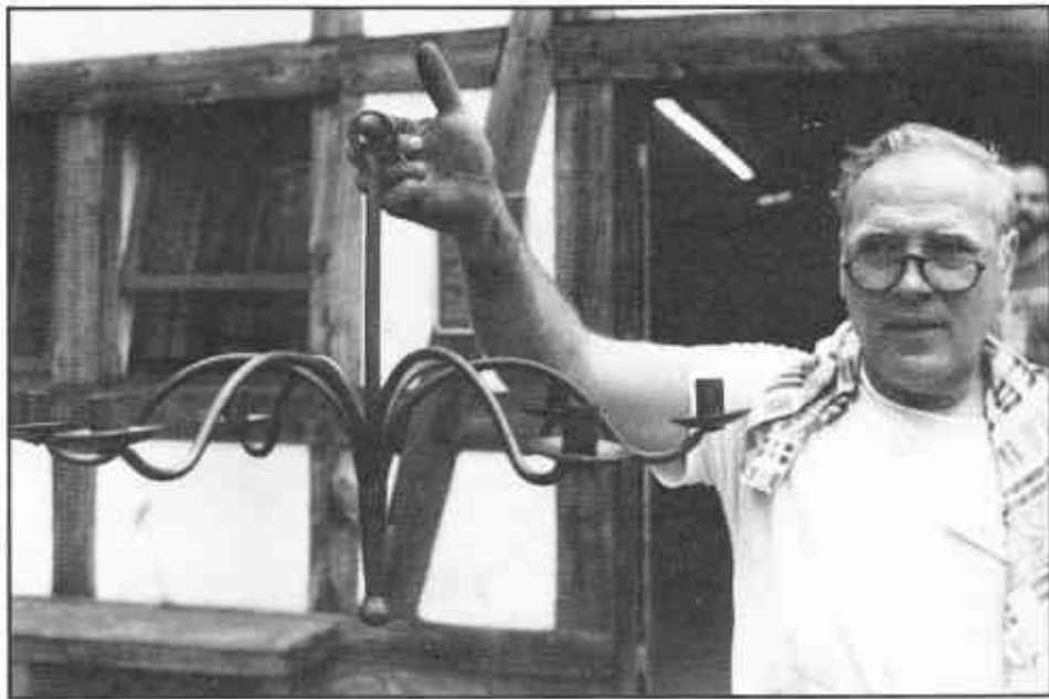
A fine chandelier made by our token Dutchman, who really didn't know what a mule is. This chandelier is a 6-arm Virginia style fixture. The center is forge welded using 6 pieces of 3/8 round wrapped around a piece of 1/2 inch round.
