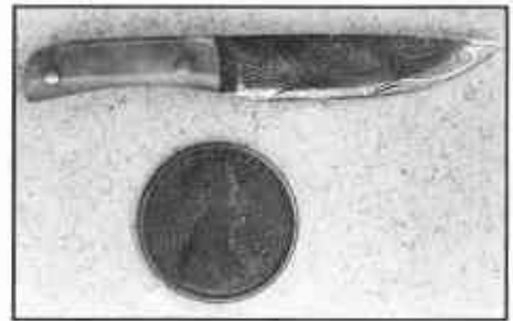
Above: A penney shows the scale of this miniature twist Damascus camp knife by V.J. McCrackin, made with 364 layers of O1 and 1018, pink mother of pearl handles n/s pins. V.J. made it for his first daughter Brittany Taylor DuLany. Photo by Kevin McCrackin.
