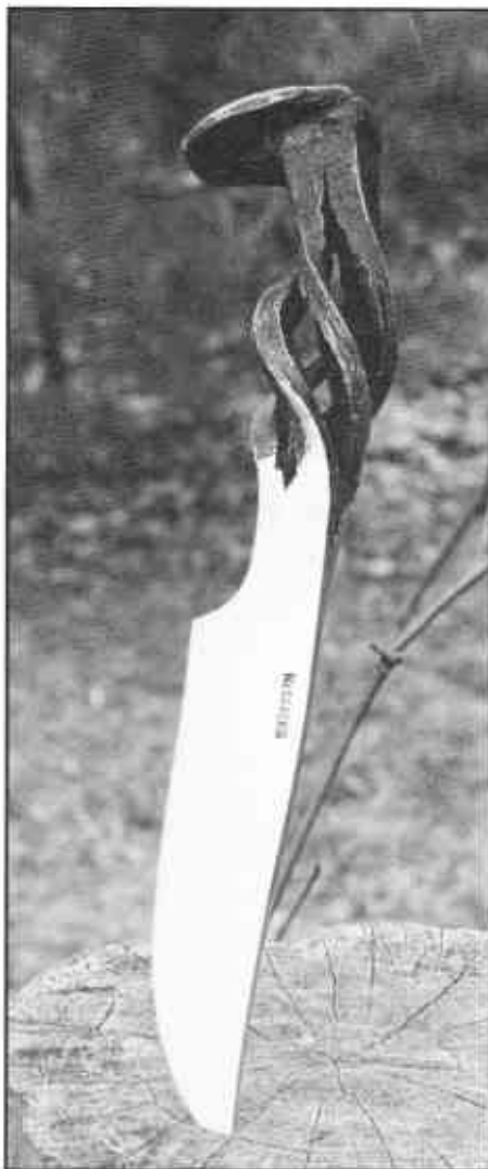
Far Left: Knife by V.J. McCrackin is 3 bar twist damascus, 203E and 1095, blade is 7 inch long sheep horn handle, nickle silver pins. Left: Railroad spike knife by Kevin McCrackin inspired by Jerry Hoffmann demo at January meeting. Handle is split four ways and then twisted. Photos by Kevin McCrackin.
