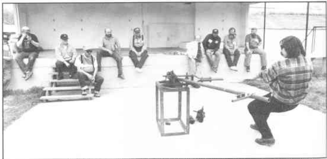
Right: ABANA President Clayton Carr shows a safe stance for using the Hossfeld bender, his specialty. Clayton made a pedal for a power hammer and donated it to the auction.
