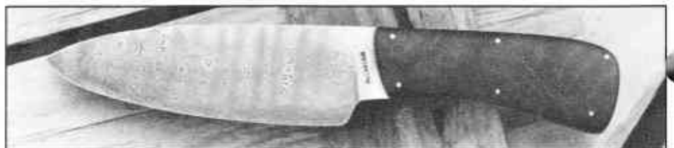
Photo #3 is a ladder pattern Damascus, 384 layers of 01 tool steel and 1018.
