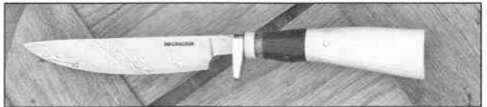
Photo #2 is a twist pattern, 320 layers of 203E and 1095.
