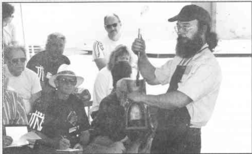
Right: Doug Wilson forges a bell from 1/8-inch plate.
