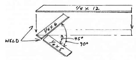
Weld the 5" and 6" piece at 90 degree thusly; the 90 degree is important.
